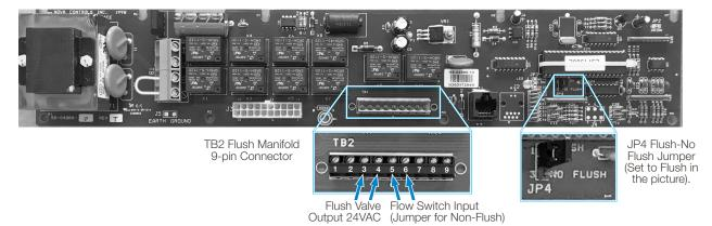
**NOTE!** In flush configurations, multiple products triggered to run at the same time will run one at a time, in queue. It is imperative that the installer allow plenty of time between triggers to ensure that a product (or group of products) will run for each of its triggers. Failure to allow sufficient time between triggers could result in triggers for products being ignored.
