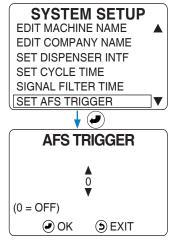
**NOTE!** Setting the AFS Trigger Signal to any nonzero value automatically enables the Auto-Formula Select feature. A setting of zero (0) will disable Auto-Formula Select.
