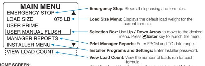
(The View Load Count menu will appear when the Selection Box is moved below the Installer Menu using the Down Arrow.)
