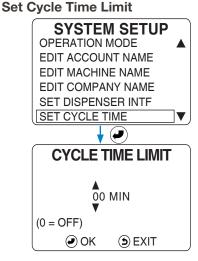
**NOTE!** The minimum non-zero Cycle Time Limit value is 30. The maximum is 99.
