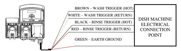
The following steps will help to insure the proper wiring of the unit. The unit should be triggered to power on from the dish machine that it is being used in conjunction with. DEMA Engineering does not recommend powering the unit separately from the dish machine. The following three steps will insure that the unit only receives power when it is necessary to have power to run the setup that is programmed in the unit.
