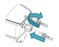
**Step 1:** Ensure there is no power to the unit, push the tube adaptors into the clamps nuts. Then tighten the clamp nuts.
