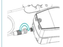
**Step 2:** Tighten the connector by turning it clockwise until finger tight.
