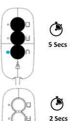
Step 1: Hold down all three buttons at the same time until the Prime indicator lights solid Blue (5 seconds)
