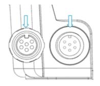
**Step 1**: Offer up the connector handset to the connector of the unit (positioned underneath the pump). Make sure the connector is lined up correctly as it will only fit in a certain position.
