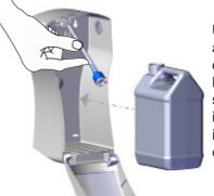
Unlock the cabinet and remove the empty jerry can. Lift the chemical suction tube and insert the tube inside the new jerry
