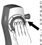
Once you have finished filling the bucket, deactivate the auto-lock function by pressing the pusher until you hear a
