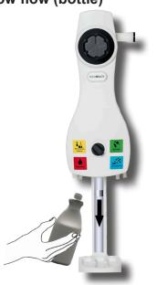
Place bottle on drip tray with the outlet tube positioned inside the bottle. To prevent foaming, there should be limited space between the bottom of the bottle and the outlet tube
