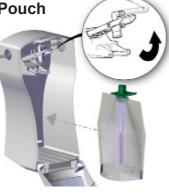
Unlock the cabinet and remove the empty pouch. Lift the pouch lever and insert the new chemical pouch
