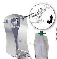
Lift the pouch lever and insert the chemical pouch
