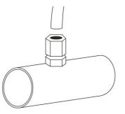
**Step 3:** Now connect the delivery tubing to the Pipe Injector, turning the compression nut clockwise until hand tight.
