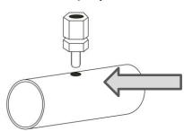
**Step 2:** For added security it is recommended to use Silicone Sealant (not-supplied) in-between the Pipe Injector and the drilled hole (as shown above). Slowly wind in the Pipe Injector until tight, it is not necessary to over tighten with tools as this may damage the threading on the injector.
