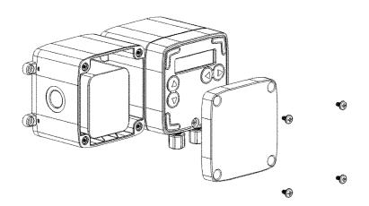
**Step 2:** Replace the x4 D Cell batteries with a high quality alkaline batteries for optimum performance and longevity. Now replace the battery holder in its enclosure and re-secure the lid.
