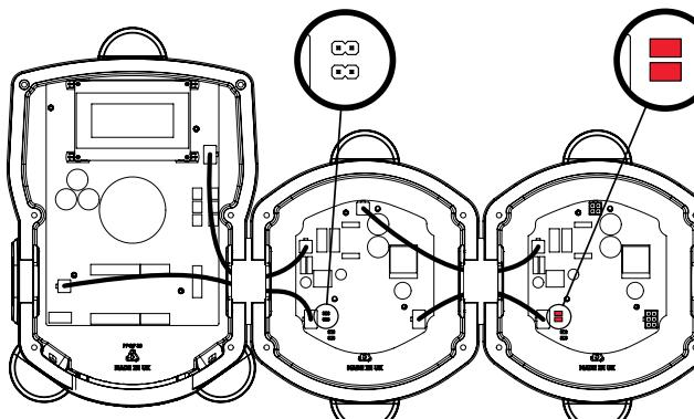
Remove the ADD ON MOTOR connector (if adding to the main board), then remove the LK3 and LK4 links, from all but the last enclosure.
