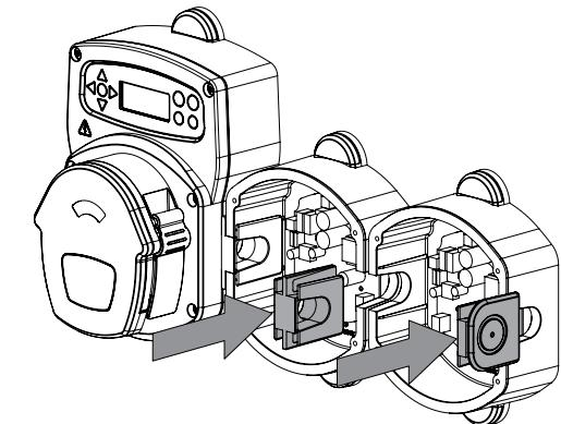
Align the Pump Module with the unit and fit the link wedge (supplied) between them, to lock them together. Then re-fit the end wedge as shown.
