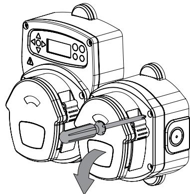
Remove the lid of the last pump enclosure, by partially removing the four screws. Carefully lift off the lid and unplug the motor loom from the motor.
