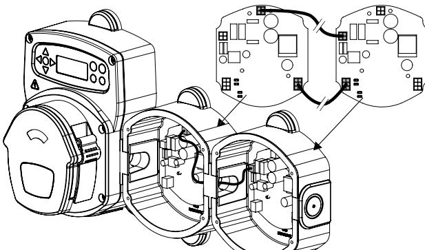
Pass the wiring looms through the hole in the link wedge, and attach them to the "MAINS OUT" / "MAINS IN" and "PORT OUT" / "PORT IN" connectors, as shown.
