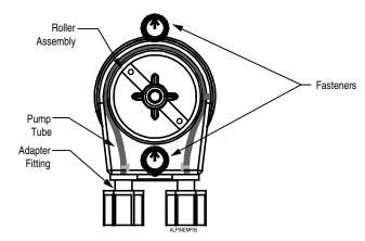
Figure 7. SnapHead Pump
