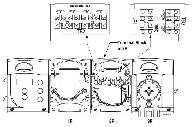
Figure 6. Alpine Wiring/Removable Terminal Block
