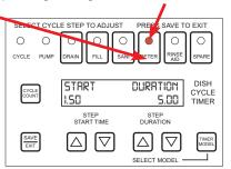
2. Change STEP START TIME or STEP DURATION using ARROW buttons (adjustments are made in 0.25-second increments).
