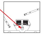
3. Wash/rinse arms are installed, secure, and rotate freely.
