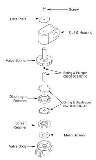
Complete 115 Volt Solenoid Valve Assembly 04810-100-53-00 Coil & Housing only 04810-200-01-18
