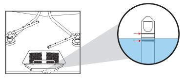
Verify drain stopper is preventing wash tub water from pouring out excessively.
