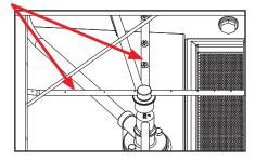
15. Ensure sump strainer and scrap screen are clean and securely in place.
