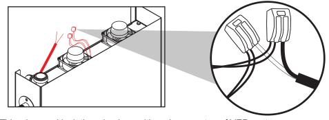
11. Tidy wires and lock them in place with p-clamp on top of VER system.
