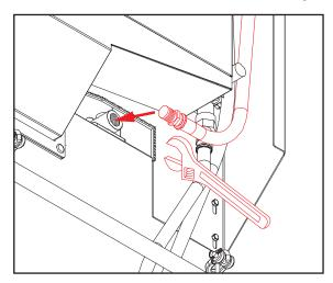
8. Use adustable wrench to connect blue hose to coupling on plumbing going to booster.
