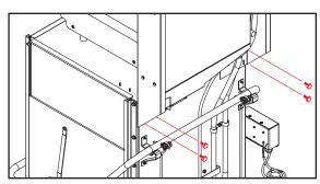
5. Use 9/16 wrench to connect gauge hose to side of tee on plumbing from booster.
