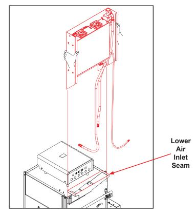
4. Install four 1/4-20 bolts located in Step 1 with 7/16 wrench.
