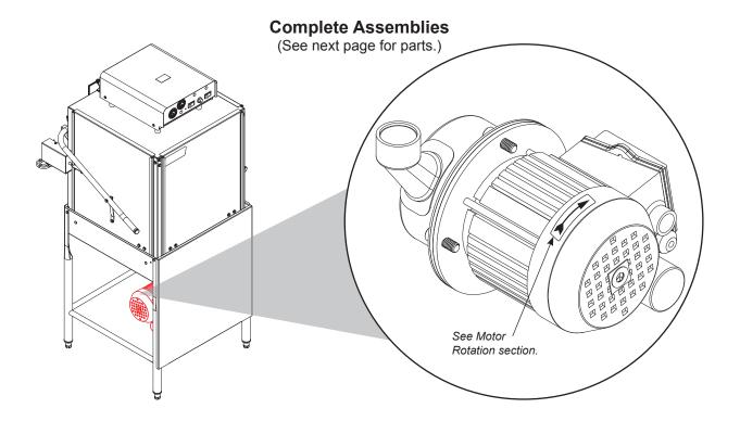
The models covered in this manual come supplied with various wash motor assemblies (a wash motor assembly includes the wash motor and the pump end), depending on the characteristics of the machine. To ensure you order the correct wash motor assembly for the model you are servicing, please refer to the following table:
