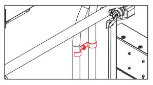
Black wire and white wire are shipped disconnected on end shown, but are already connected inside control box.
