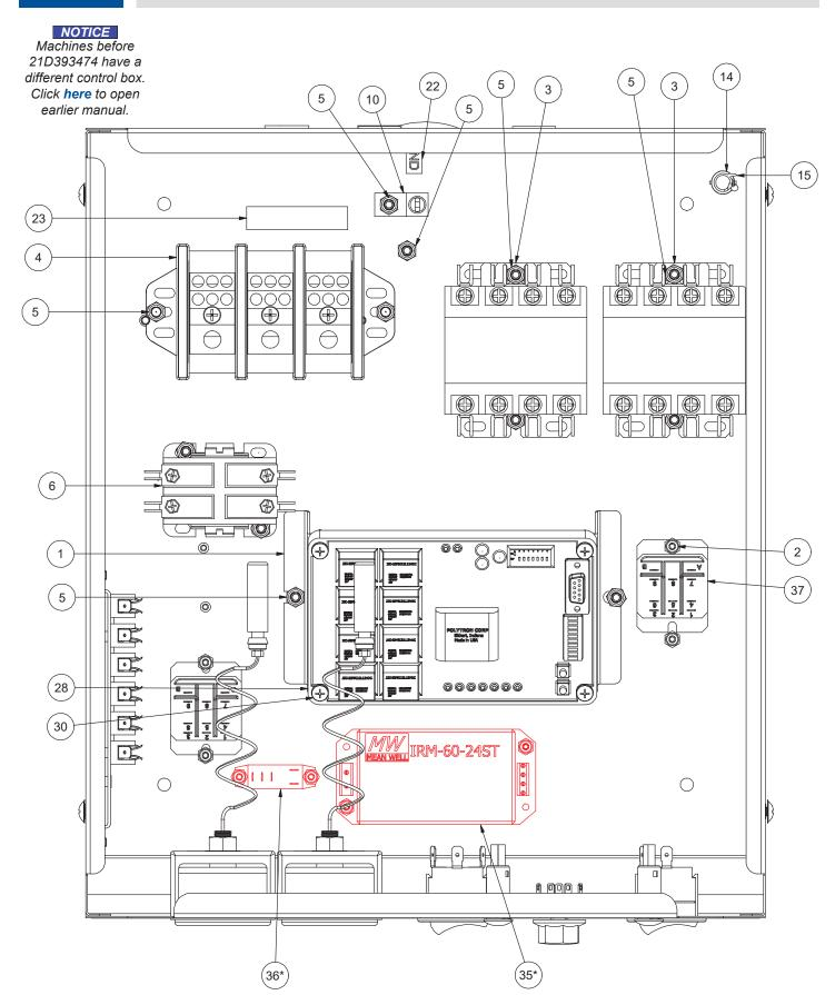
\*Power supply and relay used only on machines with door interlock and VER machines with DC fans.
