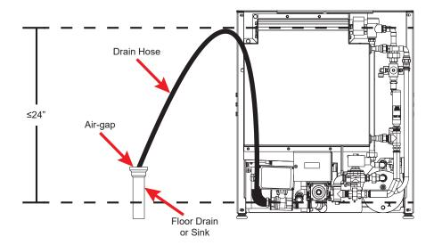
PLUMBING CHECK After installing the incoming fill line and drain hose, turn on the water supply to the machine. Check for any leaks and repair as required. All leaks must be repaired before operating the machine.
