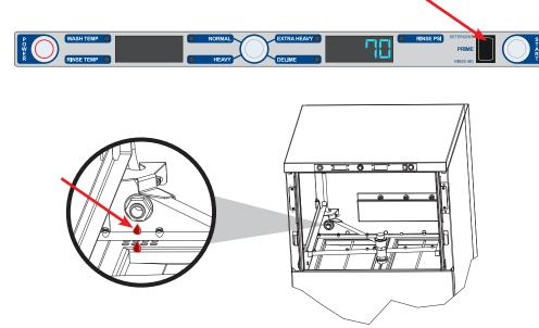
3. To prime rinse-aid pump, press and hold prime button toward "Rinse Aid" until display shows timer. Priming cycle defaults to 180 seconds.
