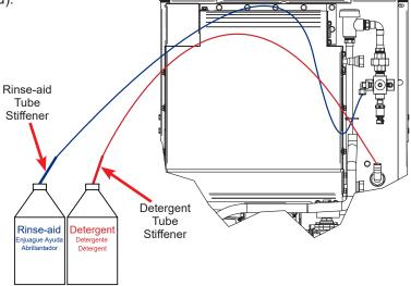
Ensure the detergent tube isn't extending past the port and into the wash chamber.
