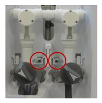
Unscrew the two screws that secure the engine to the cabinet The bucket fill and bottle fill discharge assemblies remain connected.
