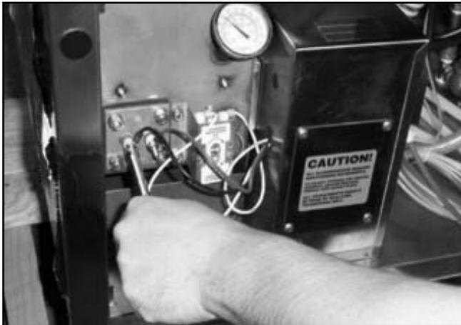
Removing the heater nuts.
