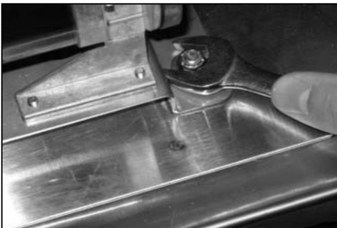
Removing the assembly mounting nuts.
