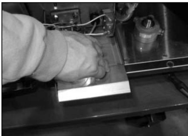
Removing the lower strainer.
