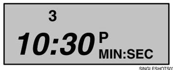
The screen above indicates that you are in program mode, in the Lockout Time Menu and have a Lockout Time of 10 minutes and 30 seconds.
