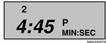
The screen above indicates that you are in program mode, in the Dose Run Time Menu, and have a Dose Run Time set for 4 minute and 45 seconds.
