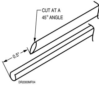
Figure 4. Cutting Chemical Feed Tubing, Inserting into Standpipe
