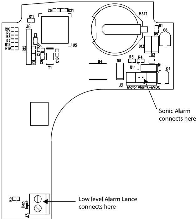
Figure 7a. Low-Level Alarm Connections
