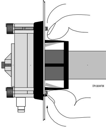
5. Remove the electrical connections at the back of the motor.
